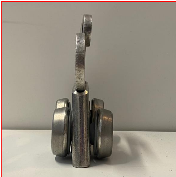
The shock absorber is twisted
