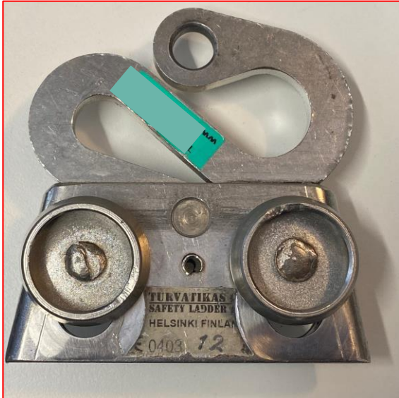
There is considerable wear on the frame
