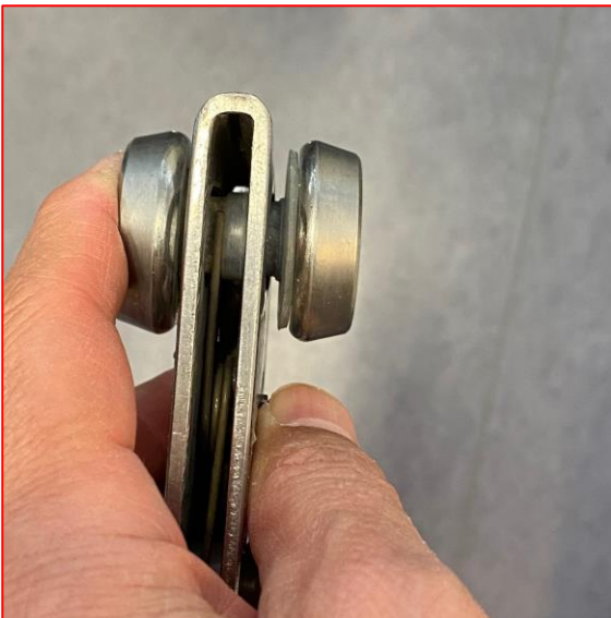
The bearings are worn out
